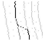
Figure 7. Tracking changes to a neighbor grain skein, since distortion pixels between the two contours lead to an error.
