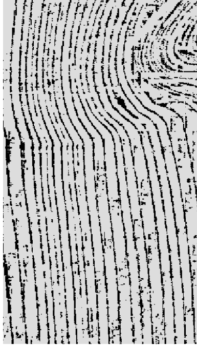
Figure 2. Grain edges detected by n-level-set-fitting: The image was divided in 10x10 rectangles. For each rectangle a 3-level-set-fitting was fulfilled and the darkest level displayed
